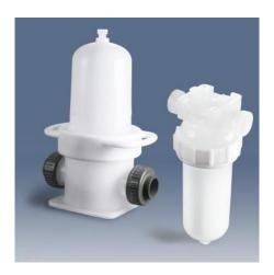
HCP Filter Housings are available in filtration media of PP, PVDF, or PFA. PP Filter Housings are suitable to filter water and regular chemicals and while PVDF Filter Housings are suitable to filter most chemicals. PFA Filter Housings are suitable to filter all chemicals hence it provides excellent temperature resistance and lower extractable; therefore is strongly recommended for the filtration of chemicals in FPD and semiconductor industries.
